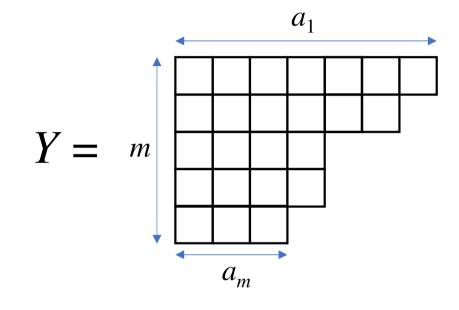
*m* rows:  $r_1, r_2, \dots, r_m$ row lengths:  $a_1, a_2, \dots, a_m$  respectively  $a_1$  columns:  $c_1, c_2, \dots, c_{a_1}$  $|Y| = \sum_{i=1}^m a_i$
